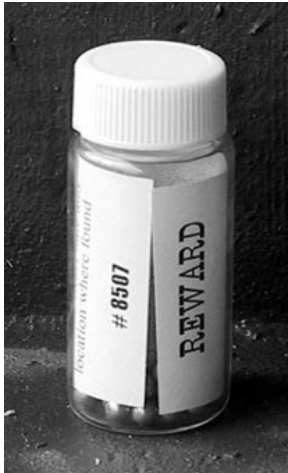
Figure 51. (Left) Drift bottle made from standard scintillation vial ballasted with BB's to the point of being only marginally positively buoyant. (Right) Locations of recoveries of drift bottles along the south Florida coast released at Riley's Hump (a spawning area) at the time of presumed spawning.
