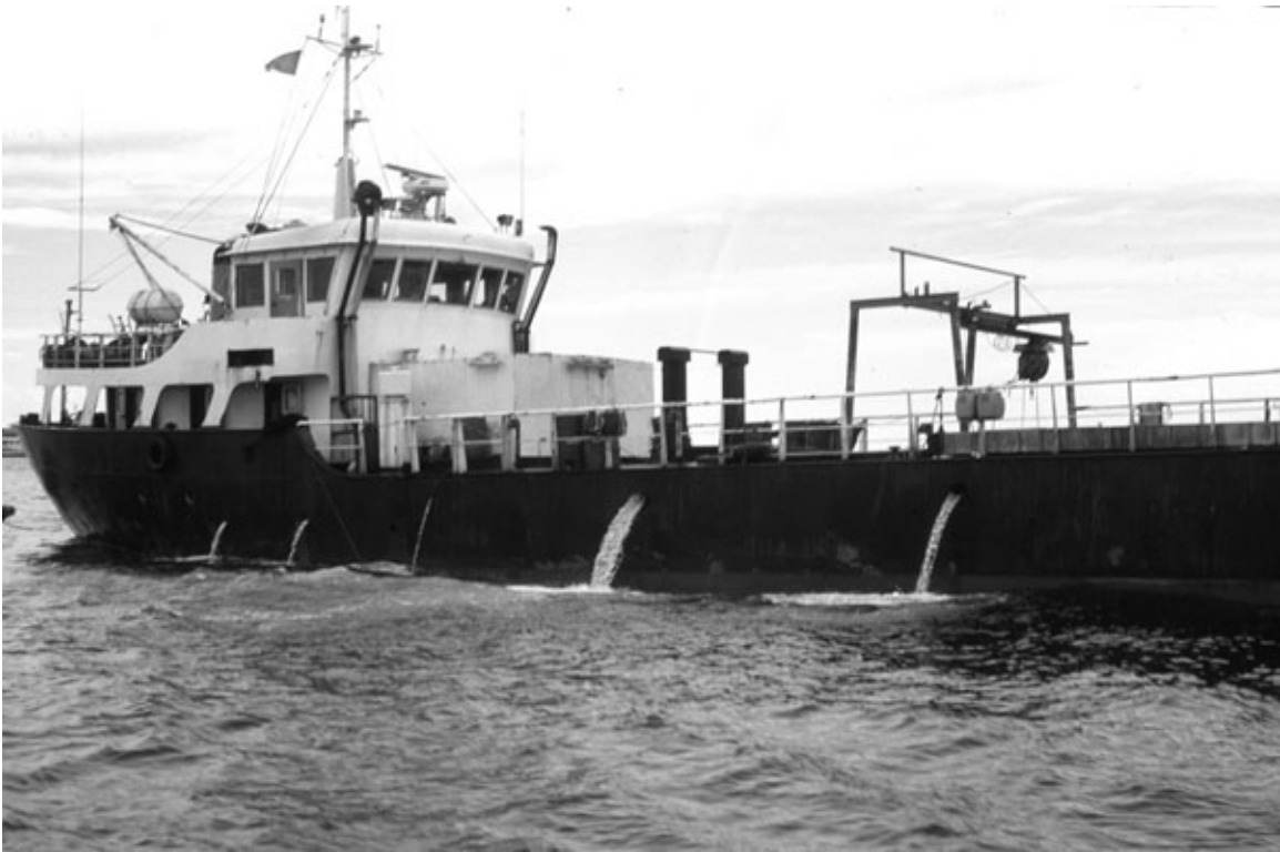
Figure 57. A Live Reef Fish Trade vessel, photographed in North Male Atoll lagoon, Maldives. Copious water pours from the tanks inside the vessel, indicative of the amount of effort required to keep its cargo of reef fish alive prior to steaming to a distant port such as Hong Kong (PLC)
