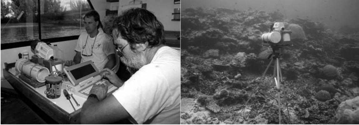
Figure 41. Autonomous underwater video system (AUVS) being programmed prior to deployment (left) and in use on the reef (right).
