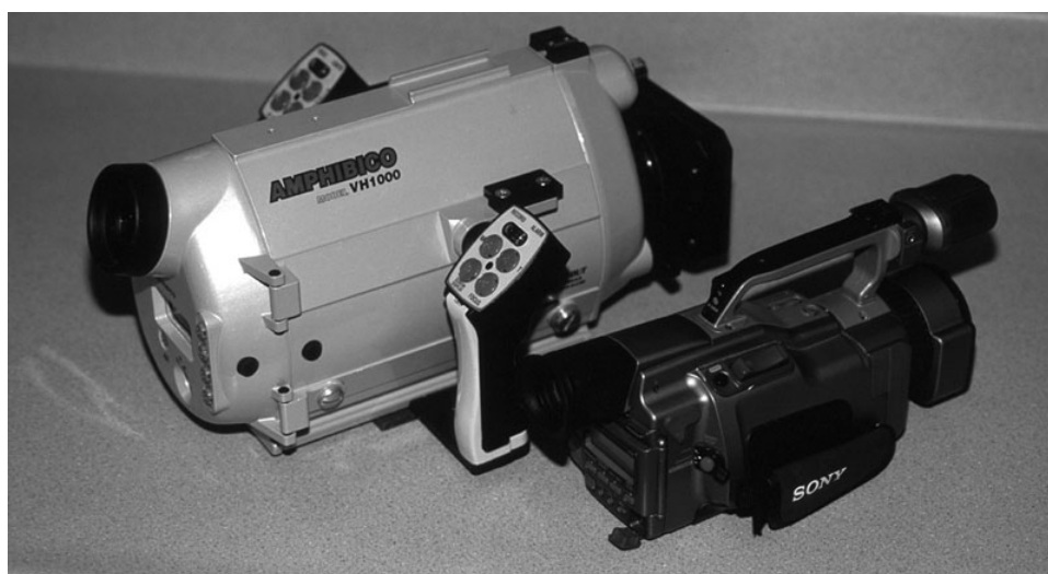
Figure 40. Typical underwater video camera with the housing on the left and camcorder on the right. This particular model, a Sony VX-1000 is a high-end three chip digital camera. It produces excellent images, but is limited in its low-light level capabilities.(PLC)
