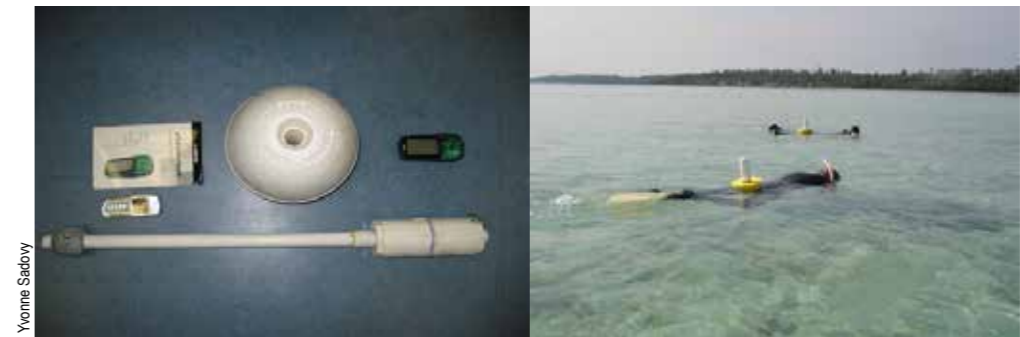
Fig. 16 Simple and inexpensive equipment enable GPS-based UVC to be conducted either snorkeling or on SCUBA on uncommon and wide-ranging species requiring long transects (Fig. 13). The GPS unit (Garmin model) is placed in a home-made PVC container that is screwed to a narrow pipe weighted to keep it upright once the buoy (white on left and yellow on right) is added for flotation.
