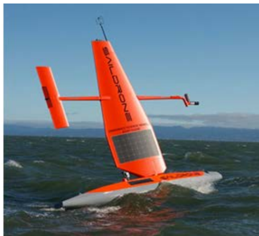
Figure 9. Unmanned surface vehicles (USVs) such as Waveglider (left) and Saildrone (right) use photovoltaic, wave, and wind energy to autonomously collect a variety of atmospheric, physical, and oceanographic data, which may be used to survey and monitor fish spawning aggregations (FSAs).
