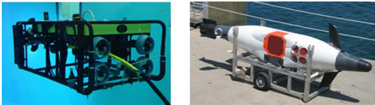
Figure 11. A high-definition, high-voltage DC remotely operated vehicle (HDHV ROV) and a Fisheries AUV (NOAA SWFSC), both equipped with acoustic, optical, and other sensors to collect data on fish distributions, species, and their sizes, and oceanographic and seabed habitats.
