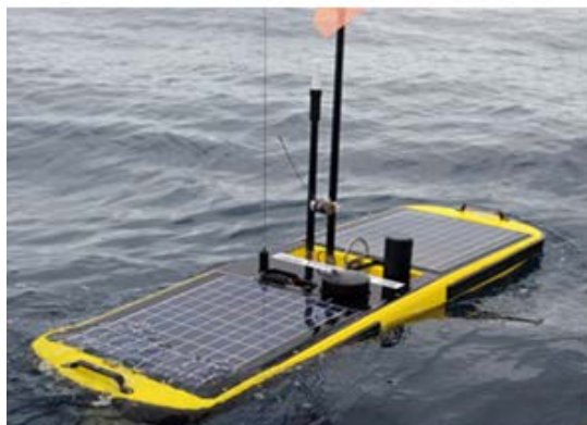
Figure 9. Unmanned surface vehicles (USVs) such as Waveglider (left) and Saildrone (right) use photovoltaic, wave, and wind energy to autonomously collect a variety of atmospheric, physical, and oceanographic data, which may be used to survey and monitor fish spawning aggregations (FSAs).
